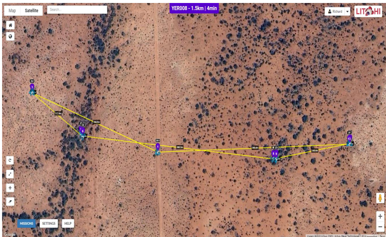
Figure 2: Flight path simulation of a monitoring site in the Litchi app for DJI drones.
