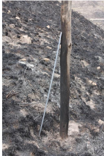
Figure 2. Example of charring on pre-planted fence post. Charring occurred higher on the leeward side of the pole.
