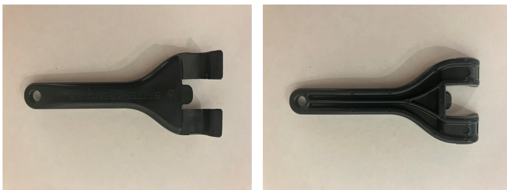
Figure 9: Battery removal tool for sheep and goat virtual fence collars. Photo credit: Flavie Audoin, University of Arizona
