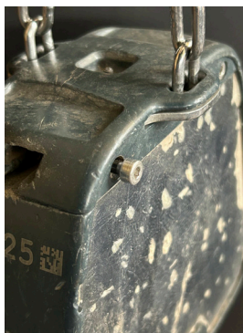
Figure 7: Hex screw that has come loose on a Nofence C2.2 model virtual fence collar. A size 3 mm Allen key for tightening bracket screws is also recommended to have on hand. Photo credit: Lara Macon, USDA-ARS Jornada Experimental Range
