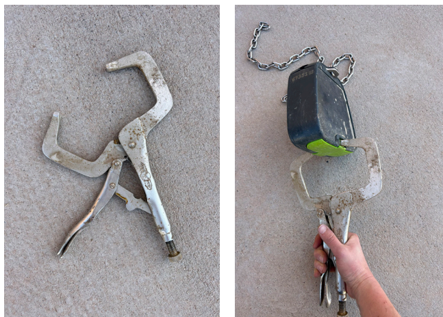
Figure 8: C style vice grips can aid in removing of batteries from many collars. Photo credit: Lara Macon, USDA-ARS Jornada Experimental Range
