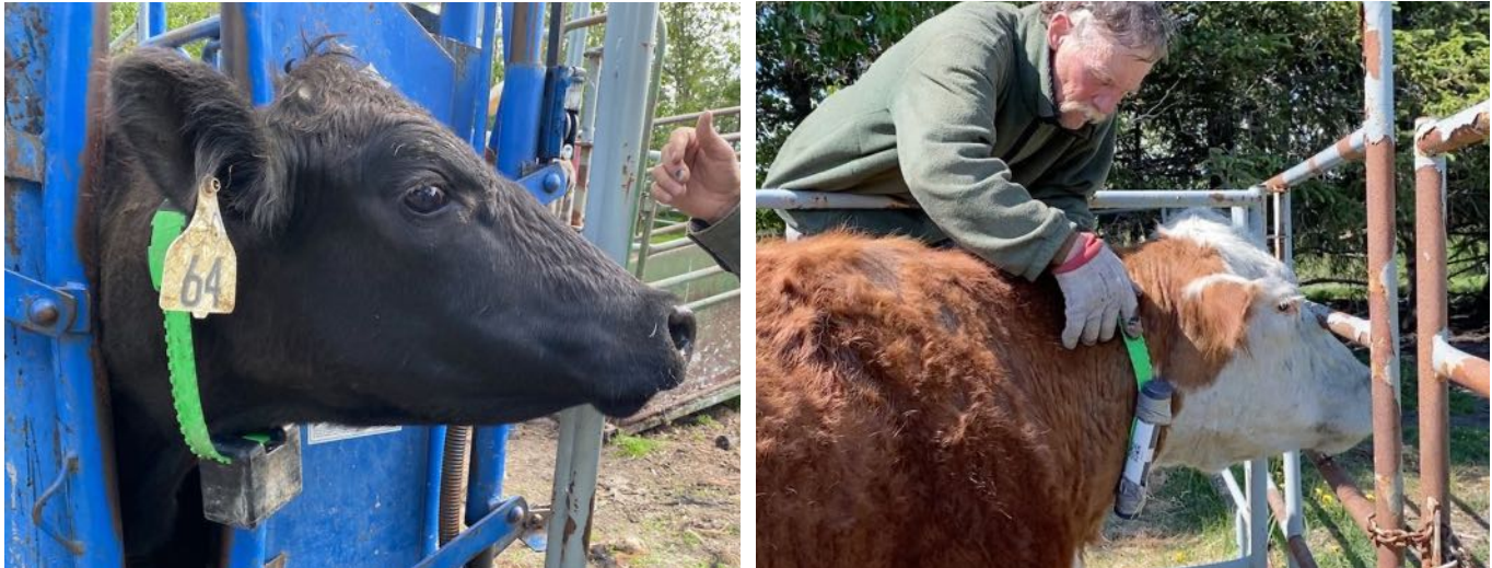
Collar-mounted GPS units in the “gateway” system mounted on cows: black box-shaped GPS unit on left, tube-shaped GPS unit on right.
