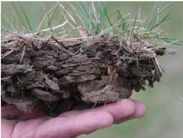
Platy soil structure in a compaction layer that is near the soil surface.
