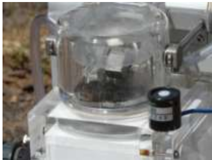
Fig. 1 Cuvette measuring chamber for CO 2 exchange of cyanobacterial crusts that remains open 90% of the time exposing the crust to natural environmental conditions.
