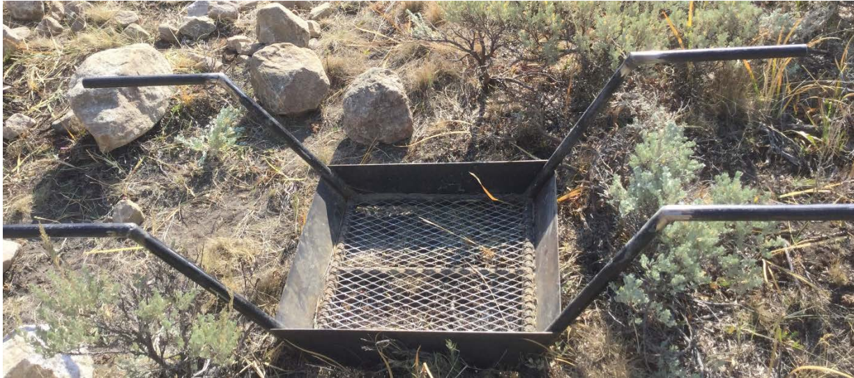
Figure 22. Steel rock carriers can be helpful tools for moving rock short distances by hand.
