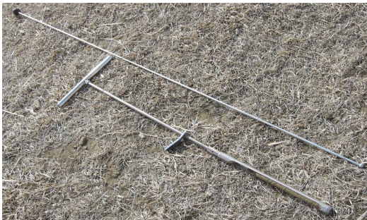
Fig. 4. Soil (bottom) and ball (top) probes are simple, but effective tools for assessing soil moisture.
