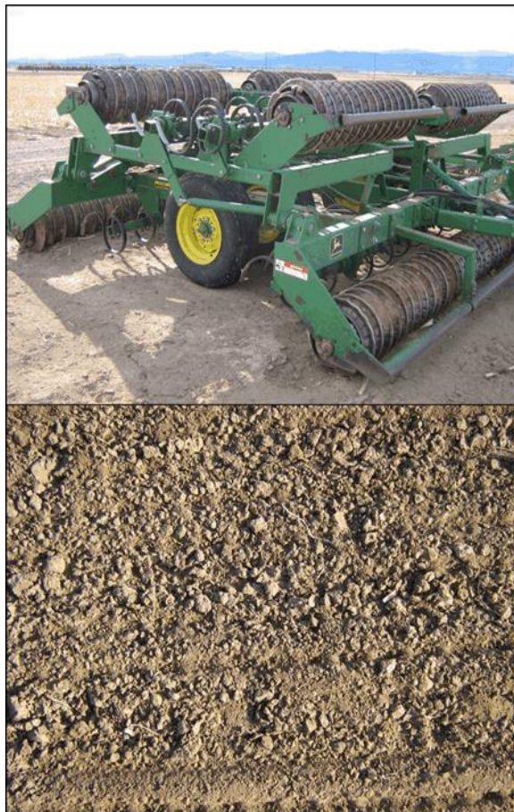
Fig. 1. Example of a cultipacker (top photo) and the firm seedbed (bottom photo) it can create prior to seeding into cultivated ground. Although a fine, firm seedbed is ideal in most situations, in this example, the soil is high in clay and it is actually good to see the small clods on the surface. If clay soils are worked too fine (i.e. powdery), they will form a hard crust following wetting from rain or irrigation which can impede emergence of many grass and legume seedlings. (Photos by Jenna Meeks and Joe Brummer)
