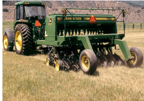
Fig. 6. A John Deere 750 no-till drill being used to interseed alfalfa into a mountain meadow. Note the rubber gauge wheels on the openers of this drill that keep the seed from being planted too deep. Unlike drills with depth bands, these gauge wheels can be adjusted so you can plant different types of seed (e.g. alfalfa versus oats) at different depths. (Photo by Joe Brummer)
