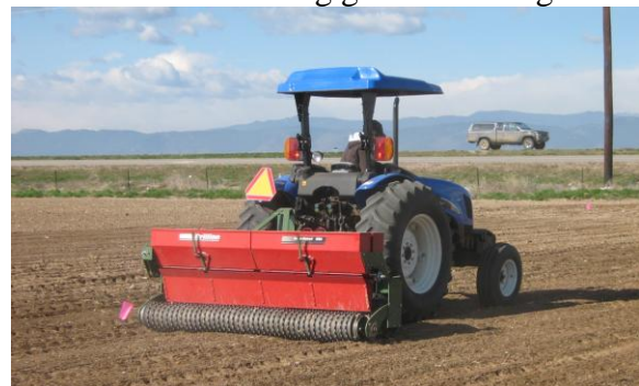
Fig. 3. A Brillion seeder being used to plant alfalfa into a clean-tilled seedbed in the spring. (Photo by Joe Brummer)
