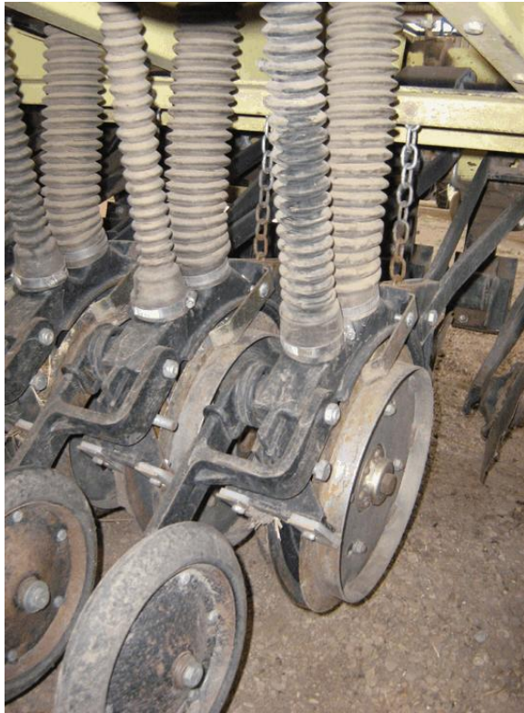
Fig. 2. Close-up of a double-disk opener with depth bands on a Truax grass/legume drill. Also, note the rubber press wheels that follow the double-disk openers and firm the seed in the soil. (Photo by Jenna Meeks)
