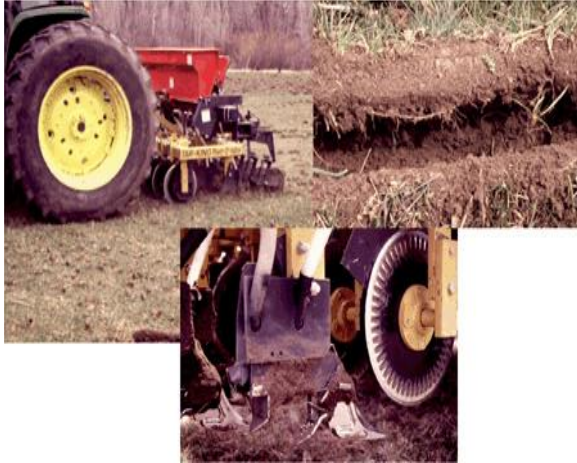
Fig. 7. A Tar-King Plant-O-Vator being used to interseed legumes into a mountain meadow. This is one of the few examples of an interseeding drill that uses a rigid shank (lower photo) to open up the existing sod. The shank is capable of placing fertilizer in the bottom of the slot, if desired, as the machine is pulled through the field. Seed is then placed shallower so that the roots grow into the fertilizer. Note that this drill eliminates some of the competition from existing plants and can create a nice, fine seedbed as long as the soil is not too moist (right photo). (Photos by Joe Brummer)
