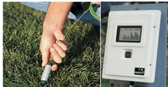
Fig. 3. Watermark™ sensor (c/o www.Gemplers.com) and accompanying Hansen™ datalogger (c/o Kimberly Research Center, University of Idaho).
