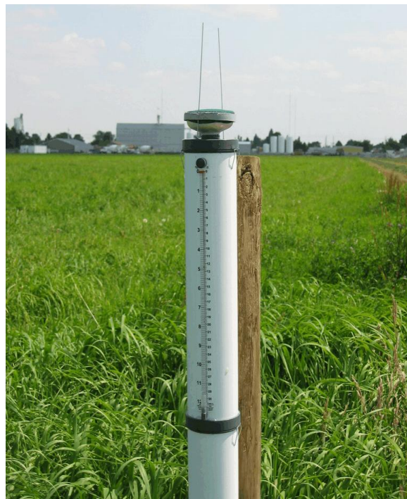
Fig. 2. Atmometer which is used to estimate evapotranspiration (ET) of grass and alfalfa hay crops.
