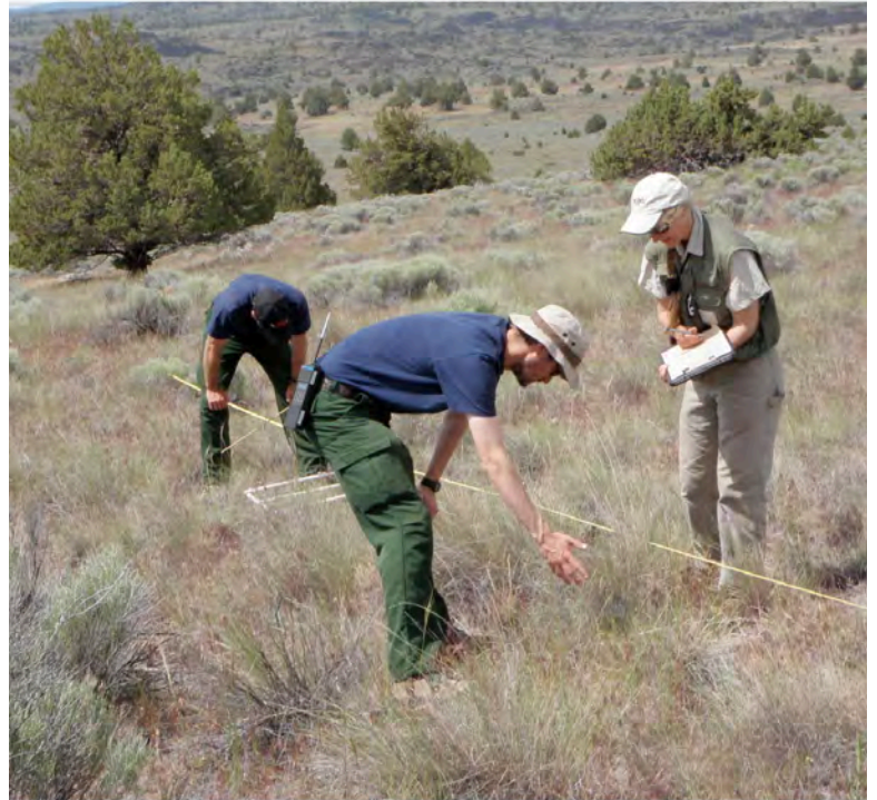
Figure 2. Sampling fuel loading using the planar intersect method at Lava Beds National Monument in northeastern California.
