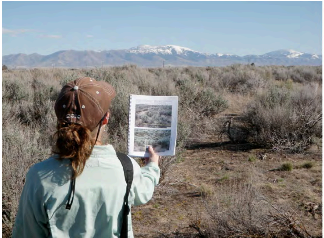
Figure 1. Estimating fuel loading on the Snake River Plain in southern Idaho using the photo series method.
