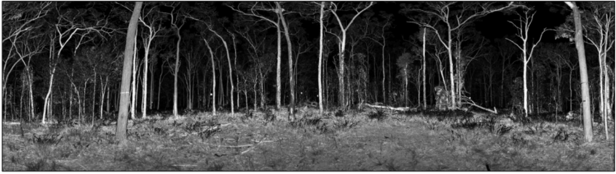
Figure 3. Example of terrestrial laser scanning of a woodland community in Queensland. The information collected is a point cloud of x, y, z coordinates enabling detailed and accurate reconstruction of the three-dimensional structure of the vegetation. The JRSRP is developing approaches with the TLSIG to derive structural metrics from these data for monitoring and accounting activities and calibration and validation of satellite-derived products.
